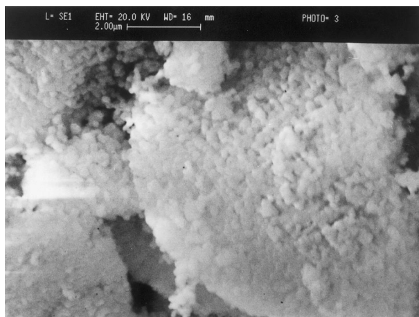
Fig. 5. SEM micrograph of the pellet sintered at 1300°C for 8 h in air.
