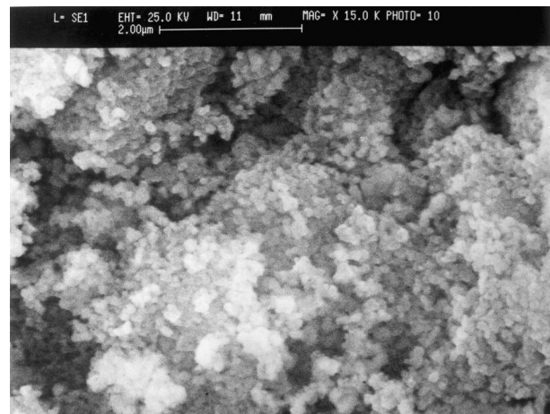
Fig. 4. SEM micrograph of the pellet sintered at 1100°C for 2 h in air.
